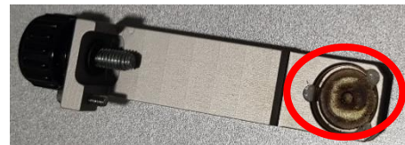
Example of damaged blast shield
